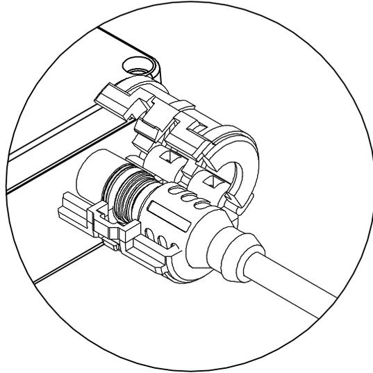
TO INSTALL LOCKOUT DEVICE, PLACE AROUND CORDSET END AND CLOSE UNTIL CONNECTOR SNAPS CLOSED. REFERENCE DIAGRAM OF CONNECTOR.
