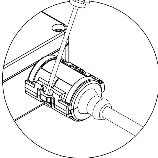
TO REMOVE LOCKOUT DEVICE, INSERT SMALL SCREWDRIVER INTO LOCKING GROOVE AS SHOWN IN PICTURE. ROTATE SCREWDRIVER IN DIRECTION SHOWN UNTIL LOCKING DEVICE RELEASES.
